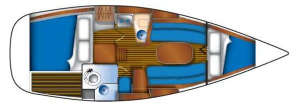
The Sun Odyssey 29.2 provides a single heads to starboard, a forepeak cabin with hatch onto the foredeck and one rear cabin. There is a chart table to starboard in front of the heads with control panel, GPS, DSC VHF radio, EPIRB and CD/radio player.
